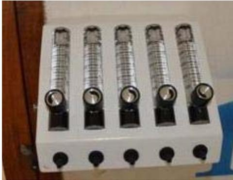
This device, made only by Airsep, splits the flow of 5L per min oxygen into five separately controlled streams in the range of 0 to 2 L per min. It is particularly useful for accurately controlling low flows to newborns and infants in the range of 0.1 to 0.5 L per min. The total flow of 5 L per min may be shared between 5 outlets. There is however the possibility of coupling 2 concentrators to 1 Sureflow if needed so that 5 patients could all have 2 L per min.
